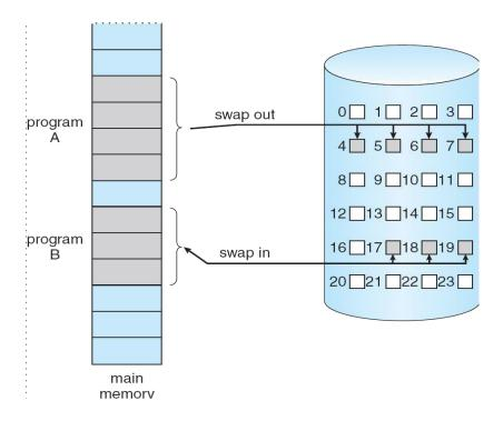
Fig. Transfer of a paged memory to continuous disk space
