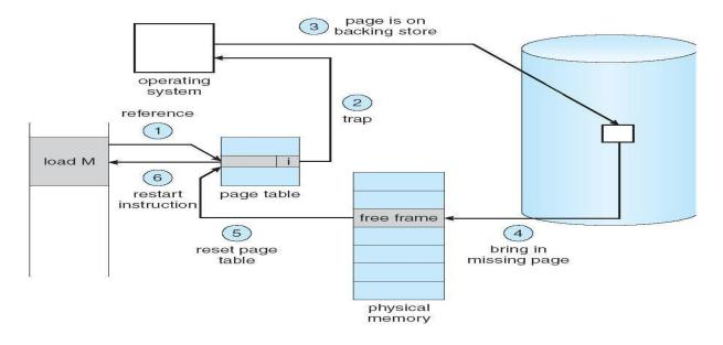
Fig. Steps in handling a page fault
